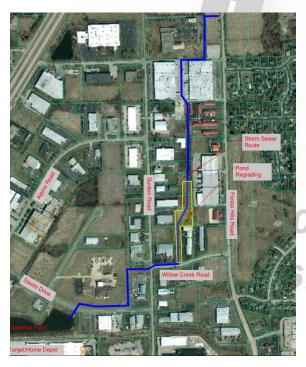
the northern end of Forest Hills Road. Once the storm sewer work is complete, the pond between Forest Hills Road and Burden Road will be regraded, and restored with new turf grass. Project limits are shown on the drawing, the blue is the storm sewer route and the yellow denotes the pond regrading.
